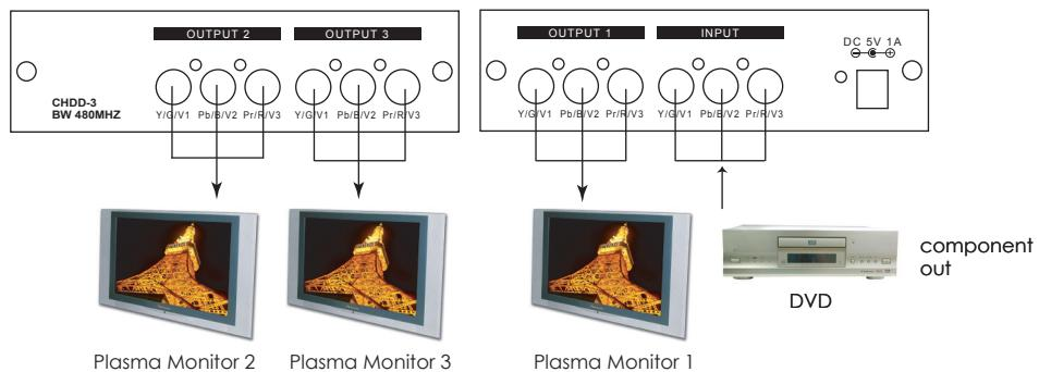
**2. Works as a 1-in 3-out distribution amplifier for HD RGsB (Sync on Green) video source.**
