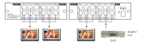
3. Works as a three 1-in 3-out distribution amplifier for composite video source.
