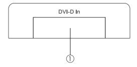
(1). DVI-D IN: This slot is to connect with source equipment such as PC or laptop for input DVI signal with DVI cable.
