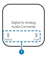
1 Coaxial/Optical Input Status LED: The LED light will illuminate according to which input is currently selected.
