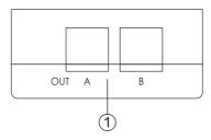
1) TOSLink (Optical Fiber) Output Ports A and B: Connect the TOSLink output ports to the TOSLink input port of audio equipments such as audio amplifier and AV receiver
