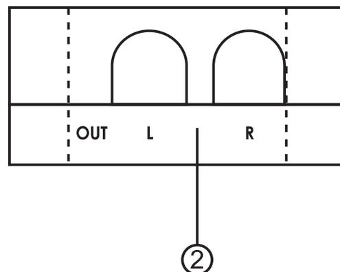
① L/R input: Connect L/R stereo analog audio input port to the L/R source equipment, such as STB.
