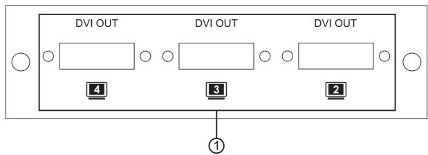
1. DVI output 2/3/4: Connect these ports to the digital input of each output display.
