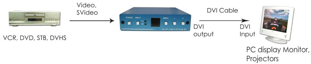
**b. Analog Out:** Connect to your TV through VGA or component interface in case your TV has no DVI input
