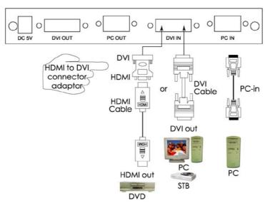
The CP-255D accepts component, PC and DVI inputs. The formats supported by these inputs are as follows:
