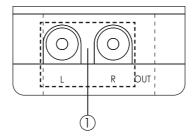
① L/R OUT: These jacks are where you connect an output stereo cable to an amplifier, speaker or TV so you can output audio.
