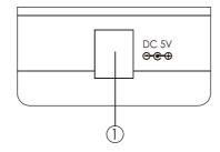
① DC 5V: This slot is where you plug the 5V DC power supply into the unit and connect the adaptor to an AC outlet.
