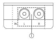
① L/R IN: These jacks are to connect with input sources such as DVD/Blu-Ray players using stereo cables in order to receive an audio signal.
