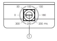
① Lip SYNC switch: This switch has eight settings that allow users to set the audio output delay from 0~300 milliseconds in order to have perfectly synched audio and video.
