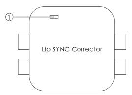
① POWER LED: The LED will turn blue when the power is connected.
