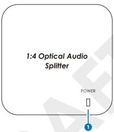
1 Power: This LED will illuminate when the unit is connected with power supply.
